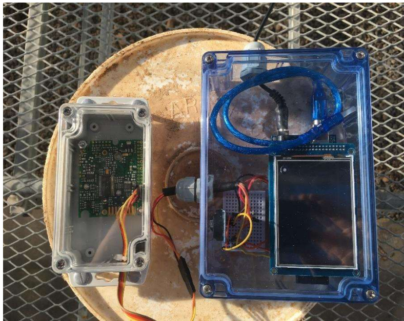
Figure 13: Custom CO 2 sensor
