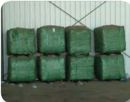
New baling equipment wraps waste in plastic before it is put in the landfill to reduce blowing litter in and around the site.
