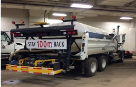
Anti-icing system on truck
